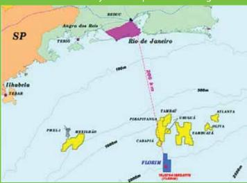
of oil and is being drilled by Odebrecht's new drillship ODN II at a water depth of 2009 meters having so far reached 5,498 meters of depth. According to Petrobras the well will continue to be drilled until it reaches 6,100 meters at which time a formation test will follow to assess the productivity of the reservoirs.
