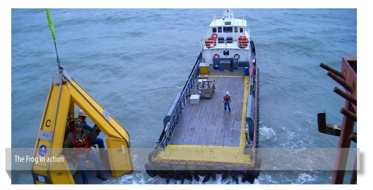
challenging. If personnel transfer offshore is necessary, it should make use of equipment with floaters such as The Frog<sup>®</sup>, instead of for instance a collapsible basket such as the Billy Pugh<sup>®</sup>.
